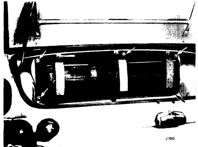
Fig. 80. Fuel tank attachment
