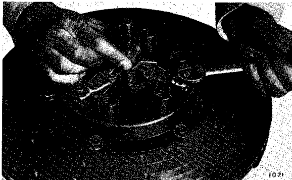
Fig. 19. Adjusting toggle height (Herald and Spitfire)
