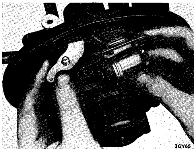
Fig. 27. Removing rear wheel cylinder
