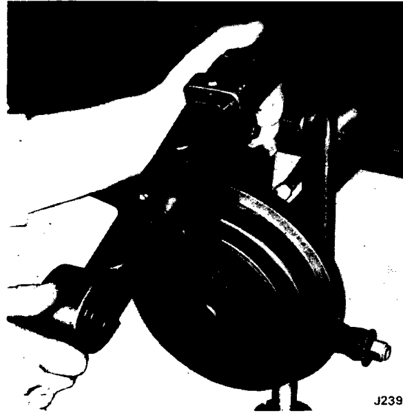
Fig. 48. Removing road spring
