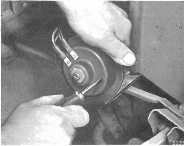
Fig. 77. Adjusting the horn
