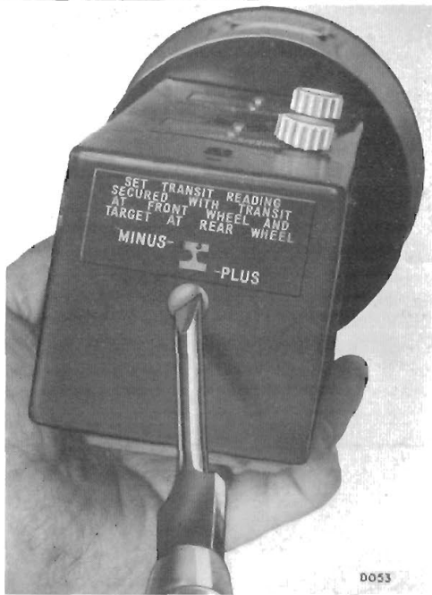
Fig. 51. Checking floor level
