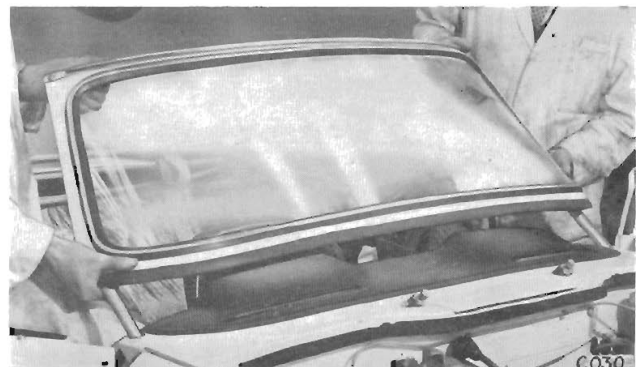
Fig. 71. Removing the windscreen
