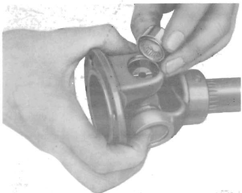
Fig. 15 Fitting cup and needle rollers
