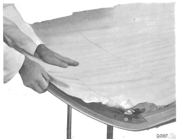
Fig. 32. Fitting front edge of lining
