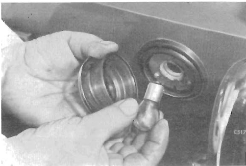
Fig. 59. Front parking and flasher lamps (Spitfire)
