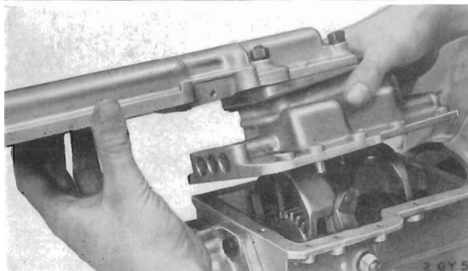
Fig. 54. Fitting top cover assembly to gearbox
