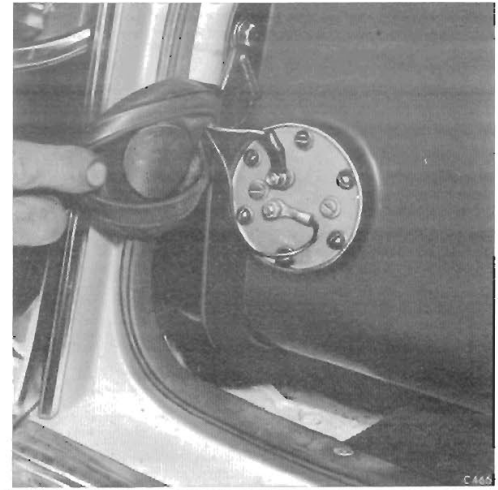
Fig. 73. Location of tank unit (Herald and Vitesse)
