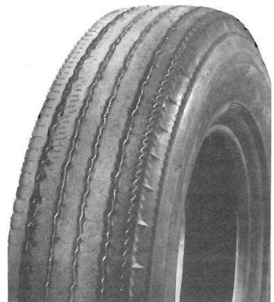
Fig. 9. Tyre wear resulting from front wheel misalignment
