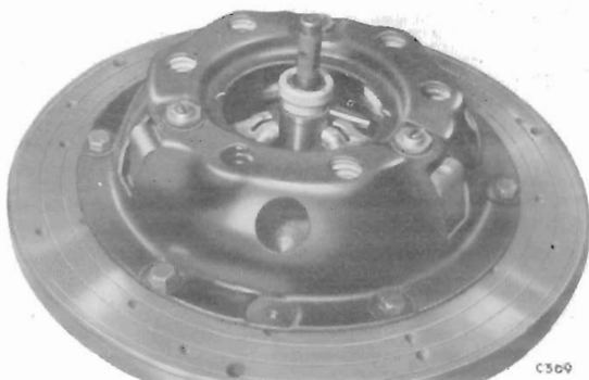
Fig. 21. Gauge finger fitted prior to adjusting toggle height (Vitesse)
