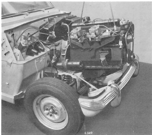
Fig. 13. Using sling to remove engine and gearbox
