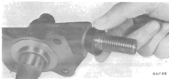
Fig. 16. Fitting rubber seal to vertical link
