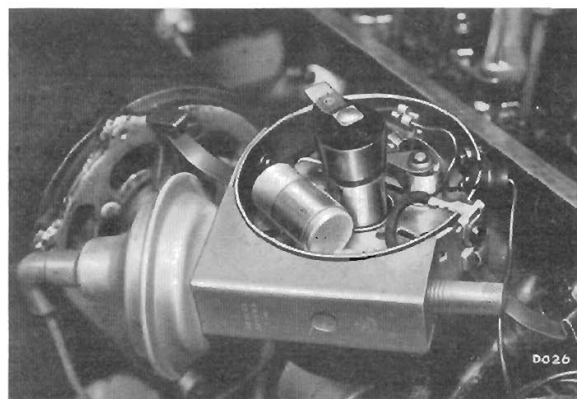
Fig. 78. Distributor rotor arm position at T.D.C. Firing on No. 1 cylinder (Spitfire)
