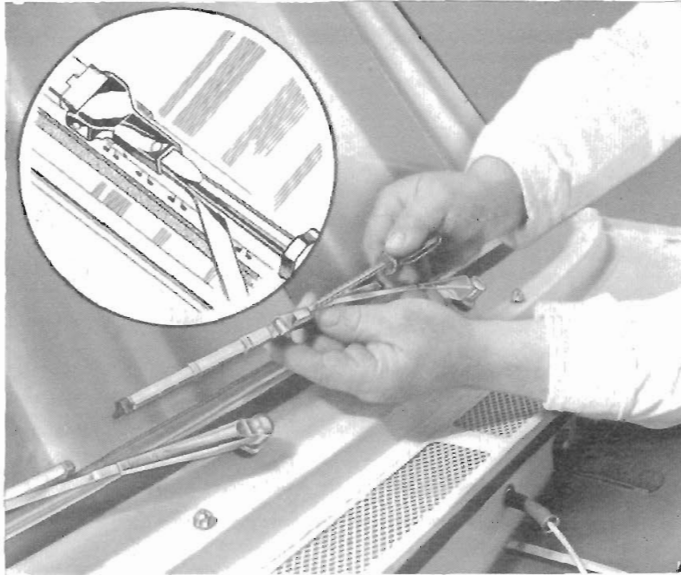
Fig. 70. Removing wiper blades
