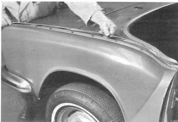
Fig. 97. Fitting wing moulding
