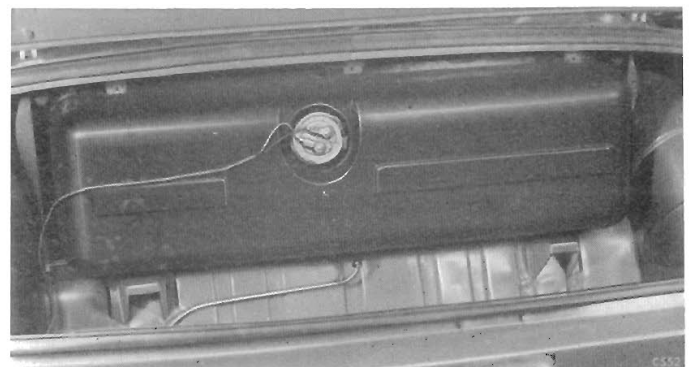
Fig. 76. Location of tank unit (Spitfire)
