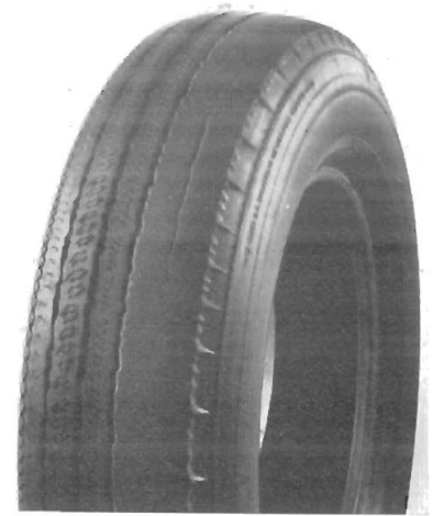
Fig. 7. The results of excessive front wheel camber
