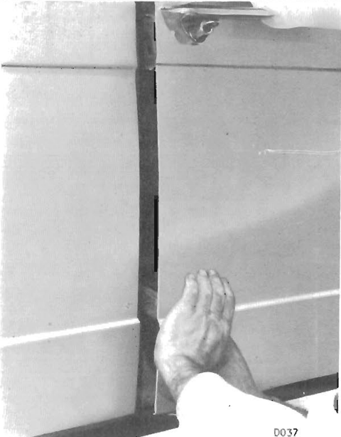
Fig. 43. Inserting wedges to increase gap
