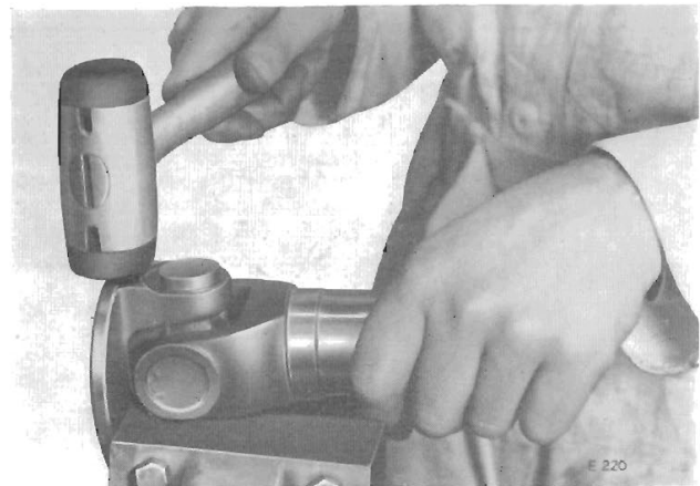
Fig. 6. Removing a bearing cup from the flange
