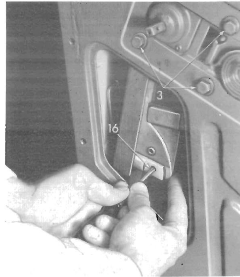
Fig. 60. Removing glass guide
