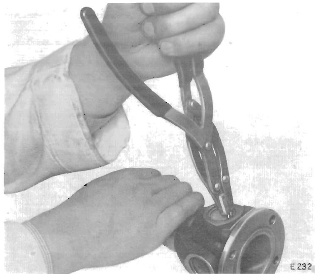
Fig. 5. Removing a circlip
