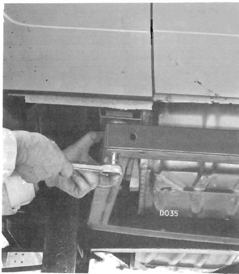
Fig. 42. Re-tightening body bolts
