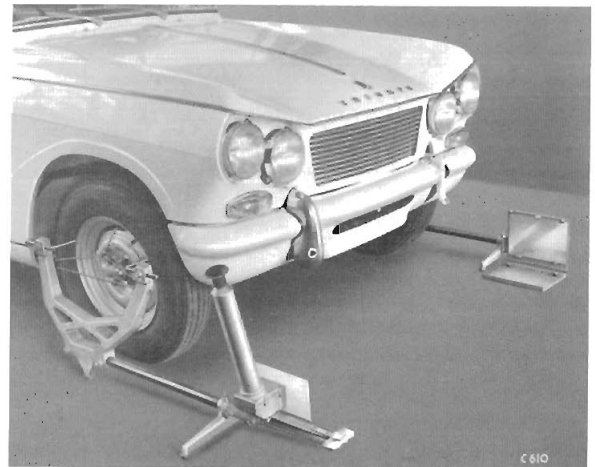
Fig. 2. Using Dunlop optical wheel alignment gauge
