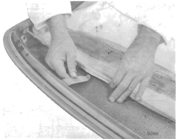
Fig. 30. Assembly No. 1 listing rail to retaining clips
