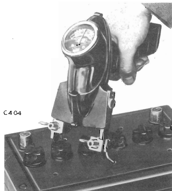
Fig. 6. Using a heavy discharge tester
