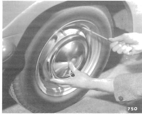
Fig. 1. Removing nave plate (Herald 1200, 12/50 and Spitfire)
