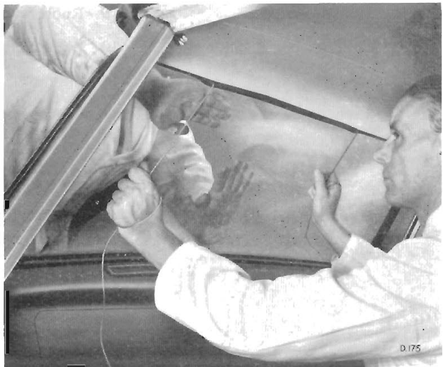
Fig. 67. Pulling the cord to turn the lip of the rubber over the body flange
