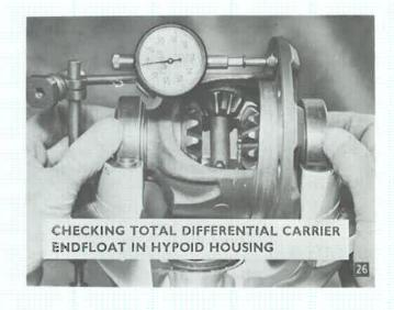
5. Before we can obtain any more figures to decide how the total shimpack should be divided between the two bearings, we must fit the crown wheel to the carrier.
