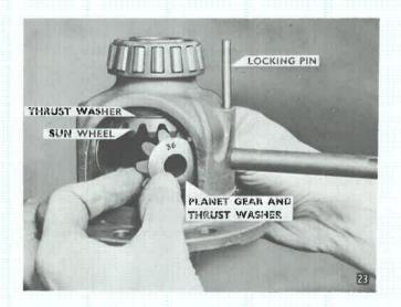
3. Finally check smoothness of gear action and if satisfactory secure cross shaft by fitting locating pin as shown.
