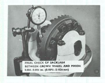
As a final check of correct meshing, paint a number of crown wheel teeth with engineer's marking blue.
