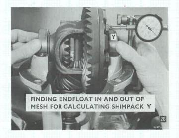
7. C. To find out the number of shims required for bearing X a simple calculation must be made.
