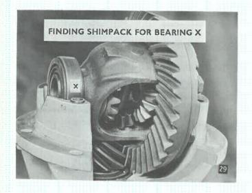
This example is to show you how to lay your figures out in order to calculate the shimpacks which locate the differential assembly into the hypoid housing.
