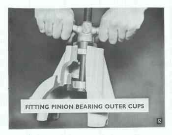
Special tools are desirable for removing the head race from the pinion. The tools shown are:-
